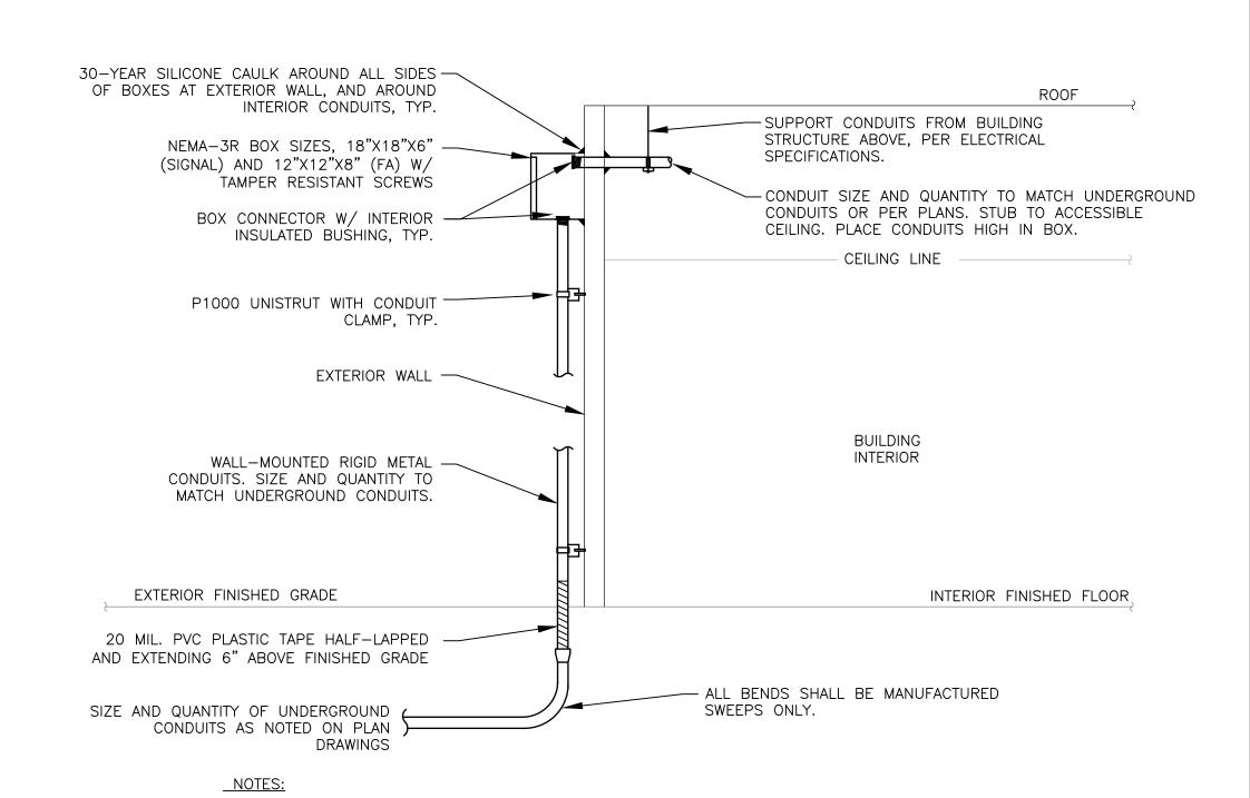
1. ALL BOXES TO BE SECURED TO BUILDING STRUCTURE USING MIN. 3/8" X 2" WALL ANCHORS/LAG BOLTS, MINIMUM 4 PER BOX. 2. 30-YEAR SILICONE CAULK AROUND ALL PENETRATIONS, BOXES AND ALL THREADS AS REQUIRED. 3. SEAL ALL UNDERGROUND CONDUITS PER COMMUNICATION PATHWAY NOTES, GENERAL PROJECT NOTES, AND PROJECT SPECIFICATIONS. 4. TERMINATE UNDERGROUND FIRE ALARM CONDUITS INTO DEDICATED FIRE ALARM BOX. ALL OTHER
