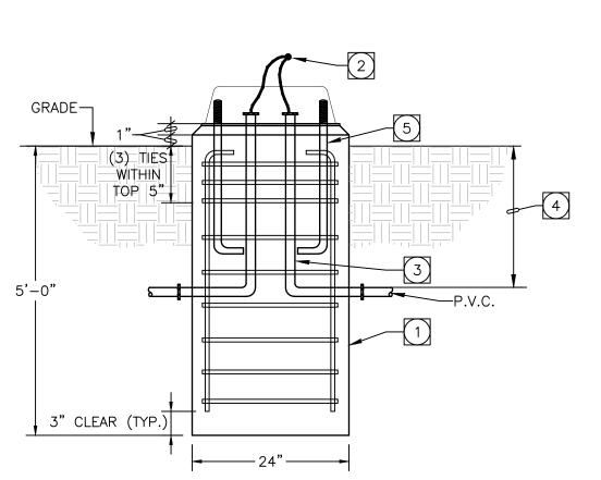
NOTE: MAX HEIGHT OF LIGHT POLE = 12'-0". MAX WEIGHT OF LIGHT FIXTURE = 35 LBS.
