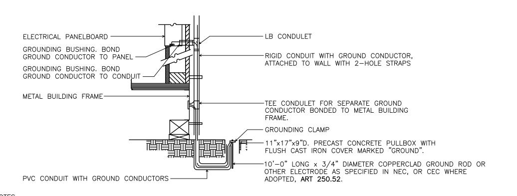
1. <u>METAL MODULAR BUILDINGS:</u> WHEN METAL BUILDINGS ARE MADE OF COMPONENTS, EACH BUILDING COMPONENT, INCLUDING STEEL RAMPS, MUST BE ELECTRICALLY BONDED TOGETHER IN A MANNER ACCEPTABLE TO DSA/SSS. PAINT ON THE SURFACE WILL INHIBIT PASSAGE OF ELECTRICAL CURRENT; THEREFORE, BOLTED CONNECTIONS OF COMPONENT PARTS ARE NOT AN ACCEPTABLE ELECTRICAL BOND.
